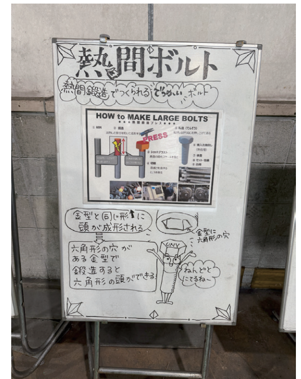
Handwritten information board explaining hot-forged bolts
