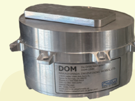
DOM1500, a deployable de-orbit device for satellites. A folded membrane measuring 1.5 meters by 1.5 meters is stored inside a compact cylindrical case approximately 10 cm in diameter and 10 cm in height.
