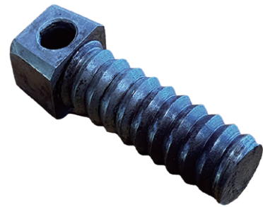
(Photo 1) A breech plug fastener fitted to the rear of a matchlock gun barrel
